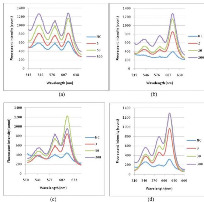
FIGURE 3. Fluorescence spectra measured from 500 to 650 nm for simultaneous detection of three target bacterial pathogens, *S. Typhimurium* (530-nm emission wavelength), *E. coli* O157:H7 (580-nm emission wavelength), and *L. monocytogenes* (620-nm emission wavelength), at 0,  $10^0$ ,  $10^2$ , and  $10^2$  CFU/0.1 ml in (a) pure culture, (b) ground beef samples, (c) fresh-cut lettuce wash samples, and (d) chicken carcass wash samples.
