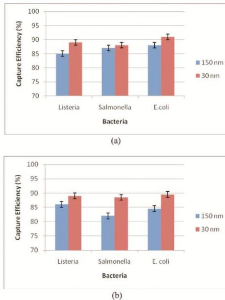
FIGURE 1. Capture efficiency for each of three target bacterial pathogens, *S. Typhimurium*, *E. coli* O157:H7, and *L. monocytogenes*, in pure culture using immunomagnetic nanobeads (MNBs, 150 nm and 30 nm in diameter) for individual (a) and simultaneous (b) separation methods. The streptavidin-bound nanobeads were coated with biotin-labeled anti-*S. Typhimurium*, anti-*E. coli* O157:H7, and anti-*L. monocytogenes* antibodies via biotin-streptavidin binding.
