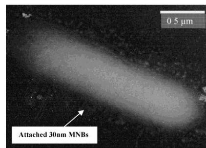
FIGURE 2. TEM images of an *L. monocytogenes* cell attached to the antibody-conjugated magnetic nanobeads (MNBs) of diameter 30 nm. The streptavidin-bound MNBs were coated with biotin-labeled anti-*L. monocytogenes* antibodies via biotin-streptavidin binding.
