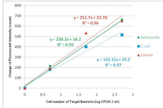
FIGURE 5. Linear relationships of the change in fluorescence intensity versus the log-transformed cell population during the simultaneous detection of three target bacterial pathogens, *S. Typhimurium*, *E. coli* O157:H7, and *L. monocytogenes*, at populations ranging from 0 to  $10^2$  CFU/0.1 ml. The changes in fluorescence intensity are the means of five replicates, and the cell populations are those of *L. monocytogenes* in pure culture.
